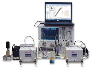
source phase, clean harmonics, wide frequency coverage from 10 MHz to 50 GHz and a flexible test set to allow the connection of ancillary components.
